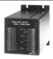
This instrument receives DC voltage and current as input signal and provides conversion output in state that the input & output is separated completely. Especially, input & output has built in photo-coupler and power, input & output have built in 3 way isolation circuit separated by transformer.
