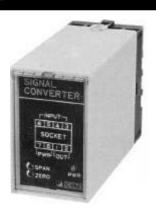
This instrument receives DC voltage and current as input signal and provides conversion output in state that the input & output is separated completely. Especially, input & output has built in photo-coupler and power, input & output have built in 3 way isolation circuit separated by transformer.
