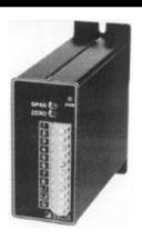
This instrument receives DC voltage and current as input signal and provides conversion output in state that the input & output is separated completely. Especially, input & output has built in photo-coupler and power, input & output have built in 3 way isolation circuit separated by transformer.
