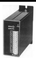
This is a high accurate converter which receives DC voltage and current as input signal and converts to reverse signal. It is possible to design loop freely by synthetic using input & output of all instruments. Especially, it is advantageous to construct loop as that input & output is separated completely and is isolated between 2 outputs.
