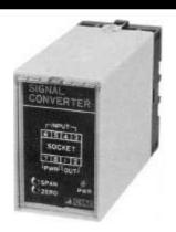
This instrument is a high accurate converter which receives RTD as input signal and converts variation of resistance following temperature to DC voltage and current output signal.
