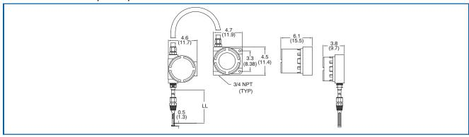
In-Line with NPT Fittings and remote NEMA 4X Enclosure – sizes 0.25" to 6"
