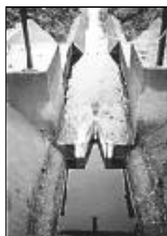
Open channel flow measurement with Two-Part system
