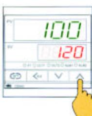
Change the set point value by using the R/S, and up/down arrow keys.
